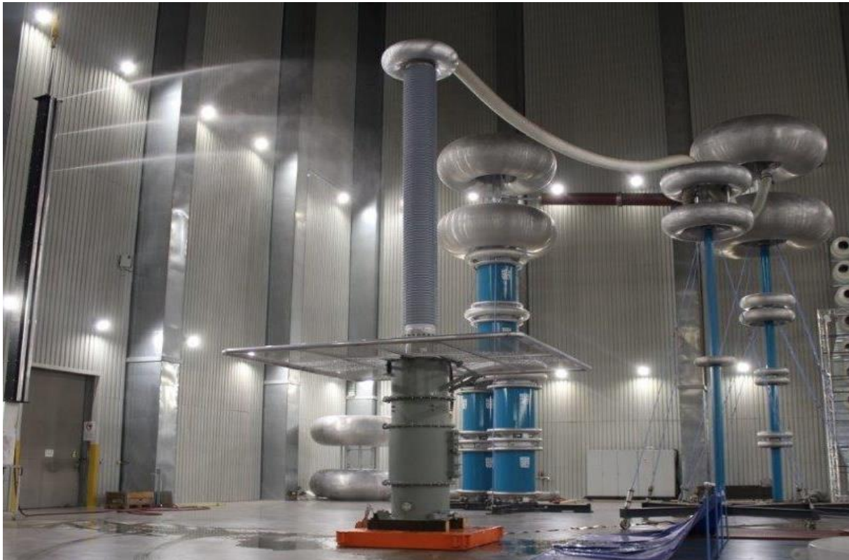
Figure 7: Type test of the 500kV RIS-HVDC bushing – Even wetting DC voltage test
