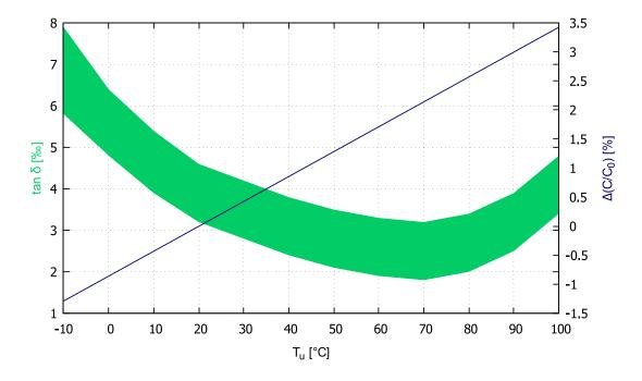
Fig. 28:  $\tan \delta (T_U)$  and  $\Delta C/\Delta C_0 (T_U)$
