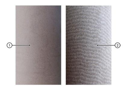
Fig. 6: Condition of the bushing
