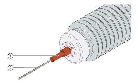
Fig. 16: Mounting the detachable conductor bolt
