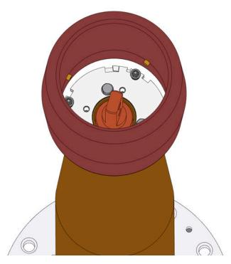
➤ To simplify mounting of the current connections, slide the electrode over the two discs on the electrode holder through the relevant apertures before putting in place.
