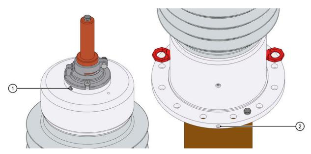
Fig. 26: Air release screws
