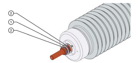
Fig. 18: Mounting the draw lead bolt / detachable conductor bolt (2)
