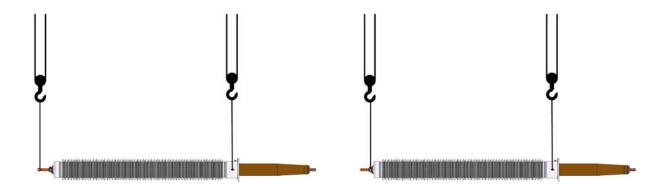
Fig. 7: Lifting with two lifting devices (example illustration)
