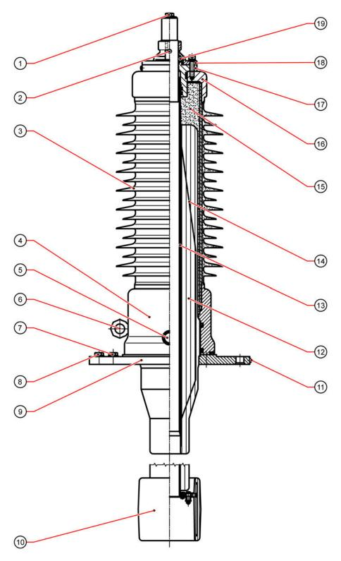
Fig. 4: Bushing design (example)
