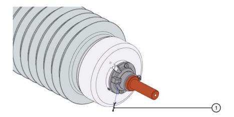
Fig. 25: Pinning the draw lead bolt / detachable conductor bolt (2)
