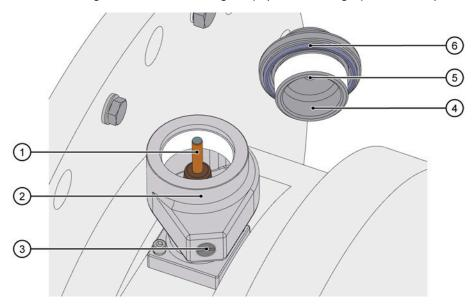
Fig. 31: Voltage tap (example illustration)
