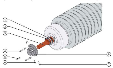
Fig. 8: Detachable parts of the bushing head
