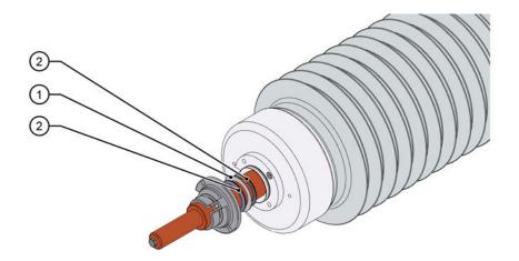
Fig. 11: Removing the draw lead bolt / detachable conductor bolt (3)
