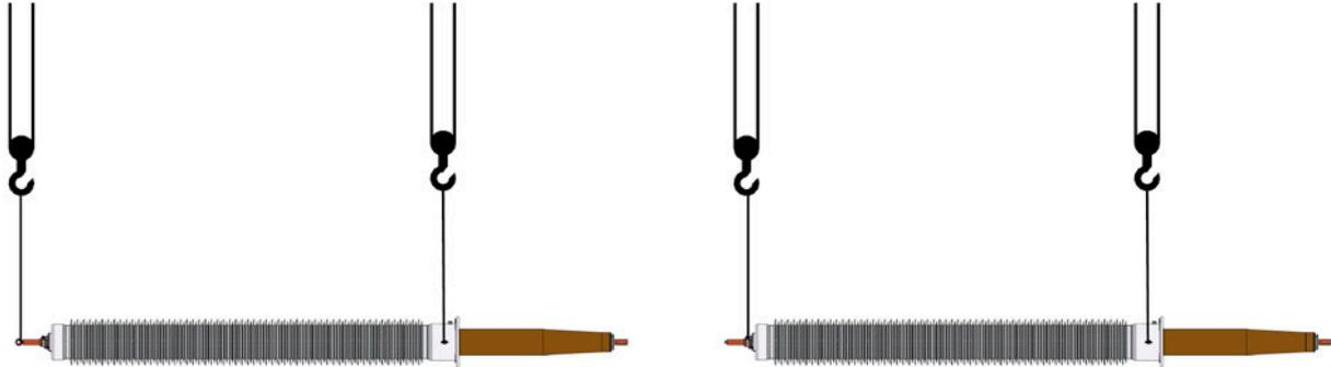
**Fig. 7: Lifting with two lifting devices (example illustration)**
