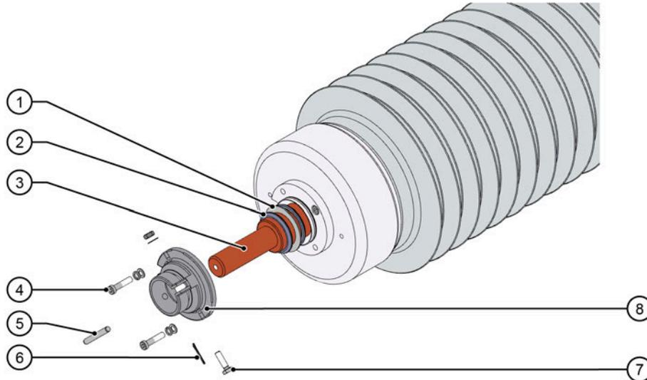
**Fig. 8: Detachable parts of the bushing head**
