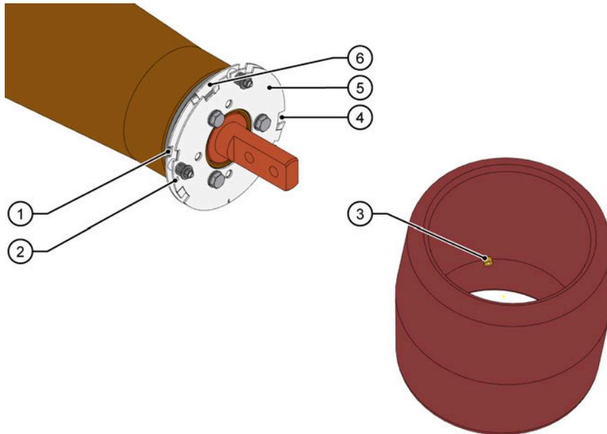
**Fig. 14: Structure of an electrode holder (here as an example with agile inner disk)**
