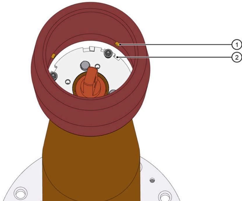
**Fig. 22: Pushing the electrode through**
