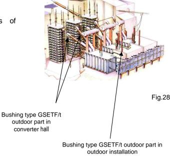
outdoor installation e.g. reactor bushing or transformer bushing in outdoor installation
